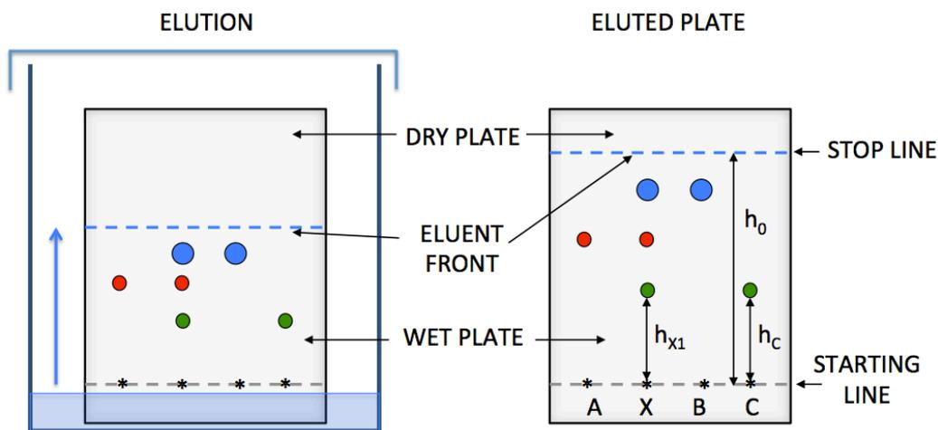
Figure 5. Separation of substances on chromatographic plate
