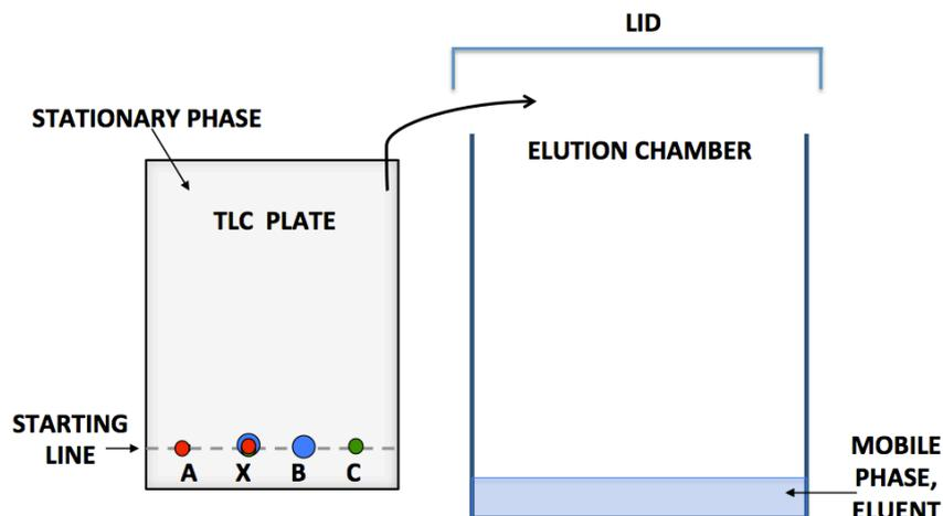
Figure 3. Spots of substances on chromatographic plate; elution chamber.
