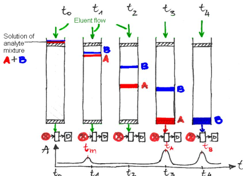
Figure 1. Principle of column chromatography and the chromatogram.
